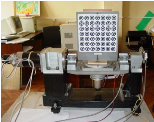
Figure 2. Calibration test field on the positioning stage
