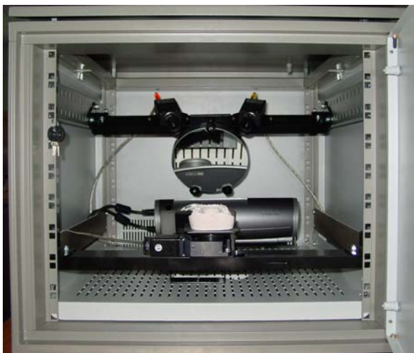
Figure 1. Photogrammetric system for teeth arch 3D model reconstruction
