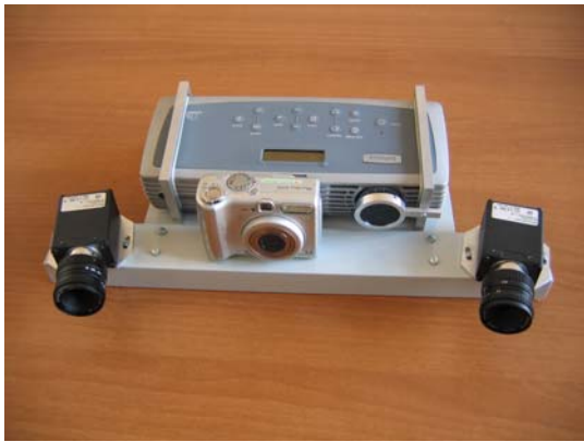
Figure3. Photogrammetric system for face 3D model reconstruction
